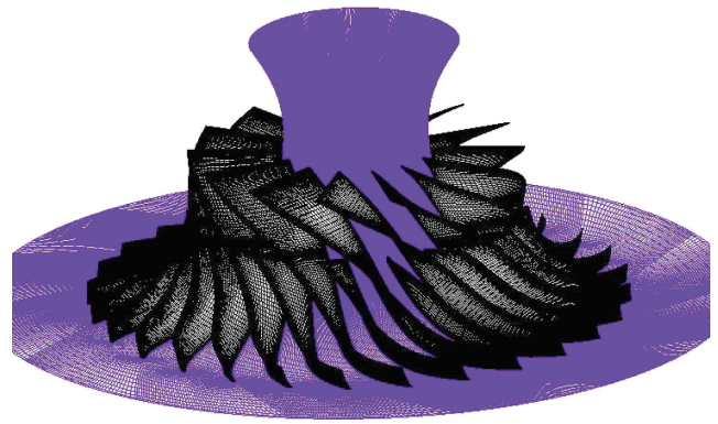
Fig. 4 Computational grid for impeller with splitter blades.
